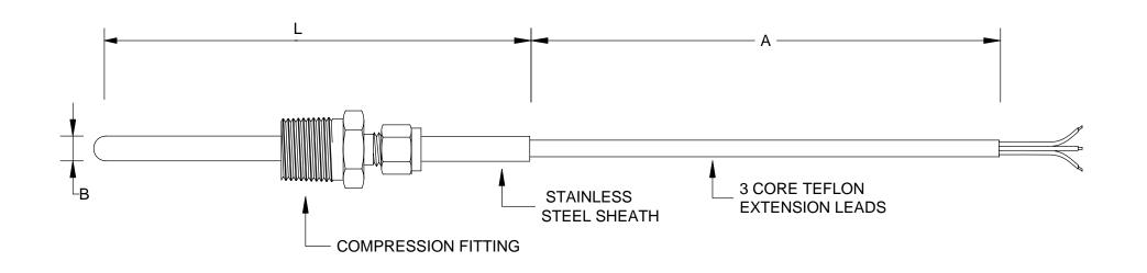
RTD PT100 SENSOR 3 CORE TEFLON TAILS AND COMPRESSION FITTING TC02 STYLE
